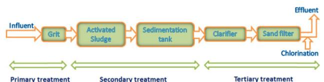
Figure 1. Flow chart of Sirte wastewater treatment plant (Sirte, Libya).
