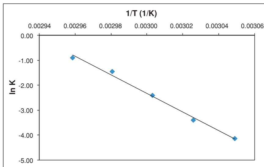
**Figure 4—Effect of temperature on the inactivation rate constant (Arrhenius model) for AAO in crushed broccoli florets.**
