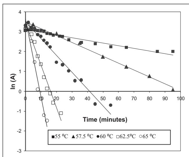
**Figure 3—Effect of thermal treatments on AAO activity (logarithmic scale) in crushed broccoli florets. Full lines (fitted curves according to 1st order kinetics model) showed the following  $R^2$  values: 55 °C ( $R^2 = 0.94$ ), 57.5 °C ( $R^2 = 0.99$ ), 60 °C ( $R^2 = 0.97$ ), 62.5 °C ( $R^2 = 0.97$ ), and 65 °C ( $R^2 = 0.98$ ).**
